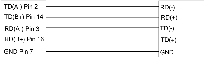
Figure 2. RS-422/RS-485 (Four Wire) Pinout Description
