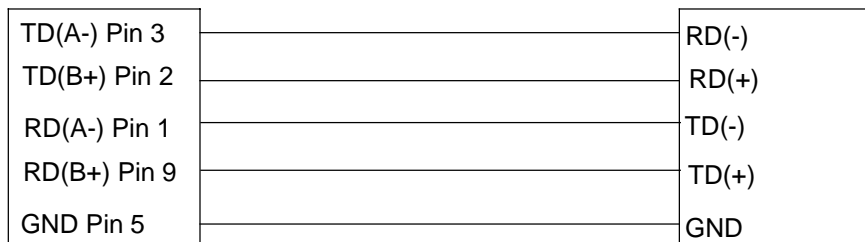
Figure 5. RS-422/RS-485 (Four Wire) Pinout Description
