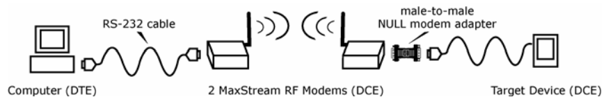
Figure 5. Example of a MaxStream RF Modem (DCE Device) connecting to another DCE device
