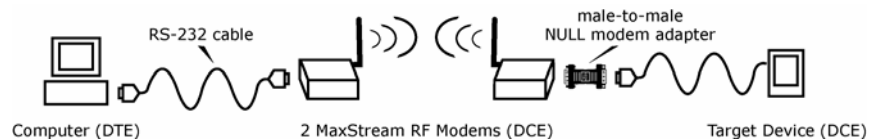
Figure 12. Typical wireless connection between DTE and DCE devices
