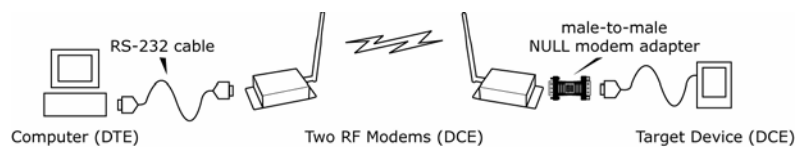
Figure 2-05. Typical wireless connection used for serial communications between DTE and DCE devices
