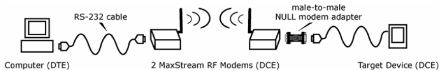
Figure B-02. Example of a MaxStream Radio Modem (DCE Device) connecting to another DCE device
