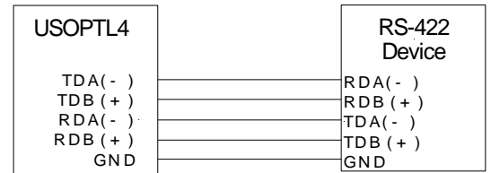
USOPTL4 in a four-wire set-up with all switches in the OFF position.
